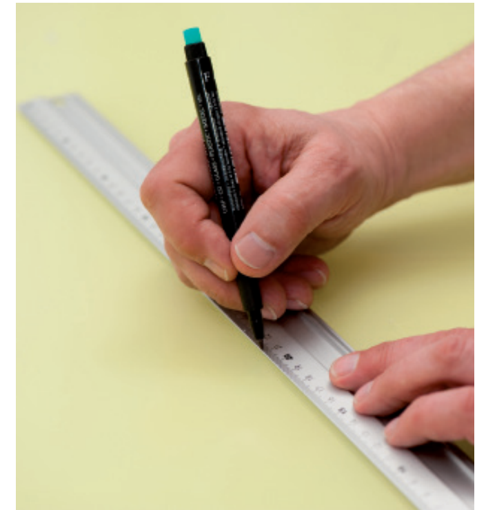
Always mark recesses and apertures on the masking film and predrill holes in the corners of cut edges.
