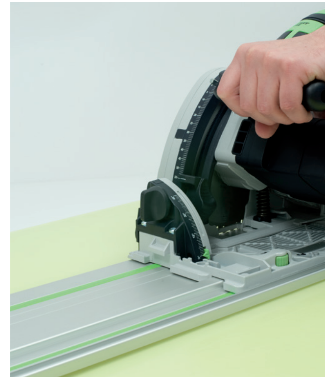
A guide rail or parallel stop is used to safely guide the circular handsaw.
