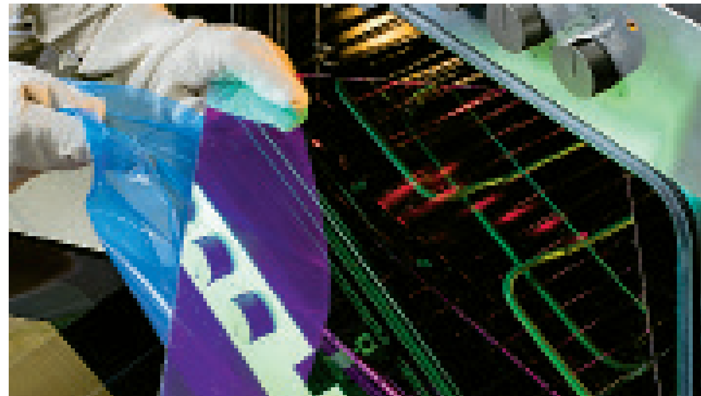
The PLEXIGLAS® sheet is placed in the airflow oven without its protective masking. Wear gloves to remove the sheet from the oven!
