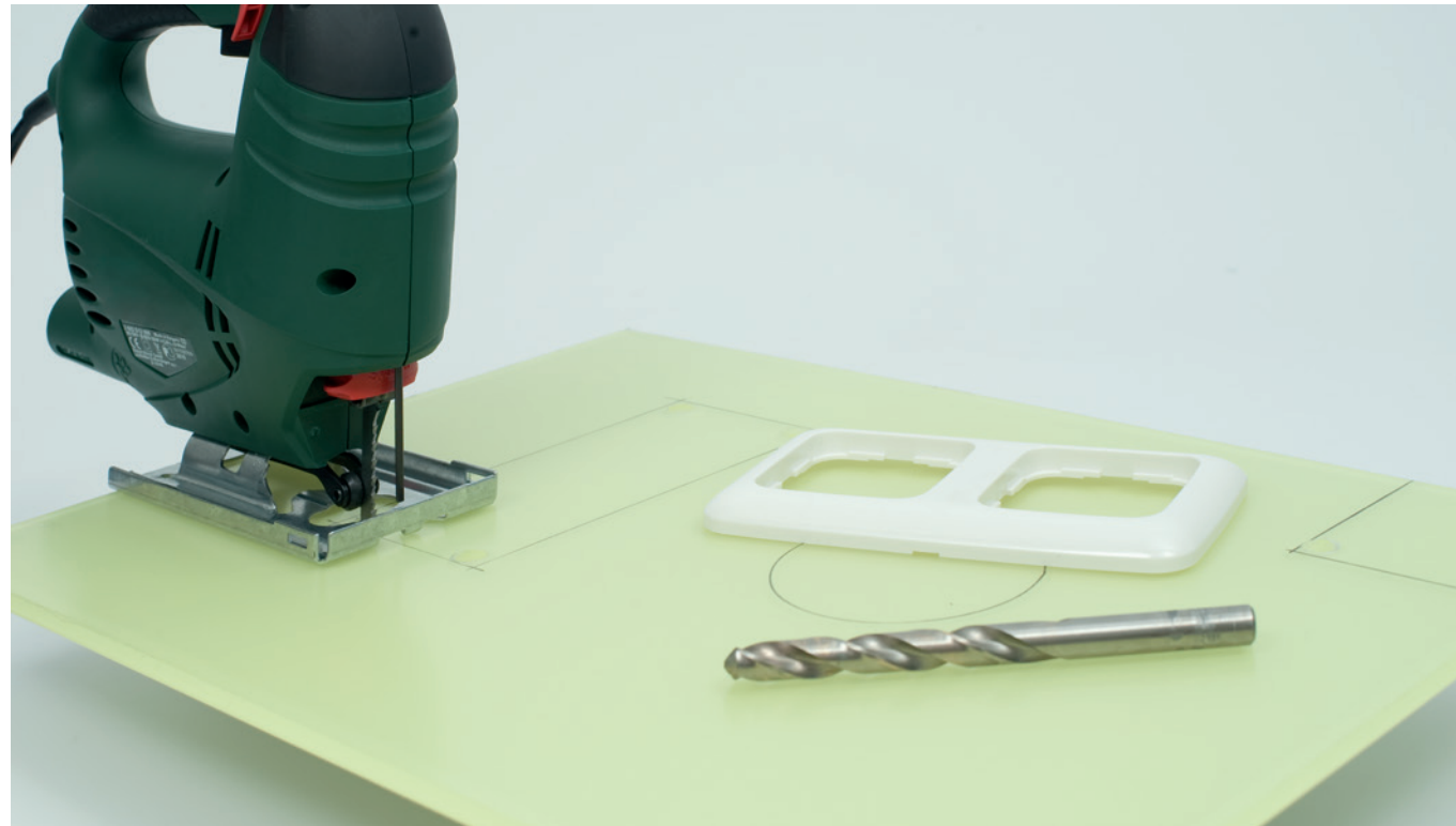
Always predrill recesses and apertures in the corners of cut edges and cut them out with a jigsaw or overhead template router.
